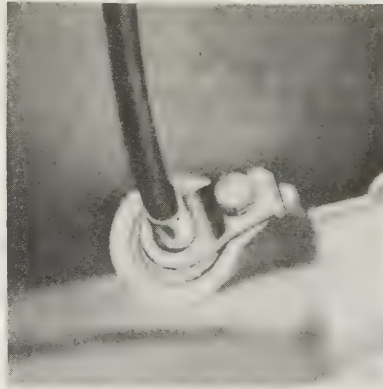
Fig. 6.14. Speedometer cable retaining clamp (Sec. 11)
