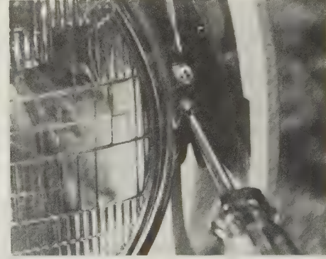
18.2 Removing the headlight unit retaining screws (the screw above is the adjusting screw)
