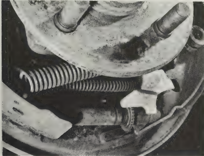
9.32A Adjustment lever correctly fitted
