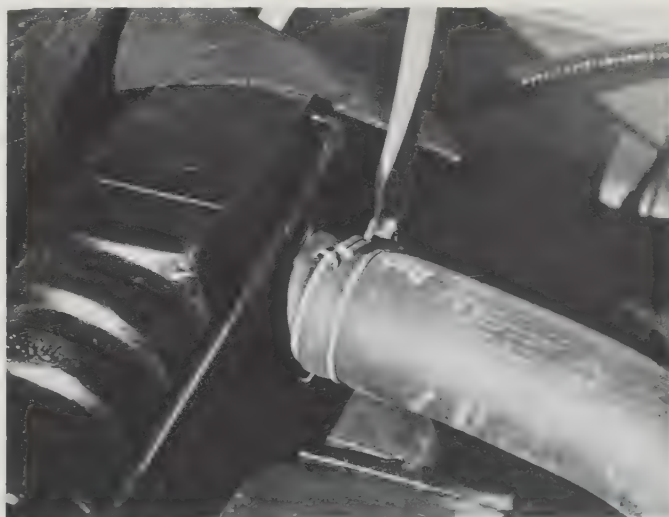
5.2 Removing top hose clamp
