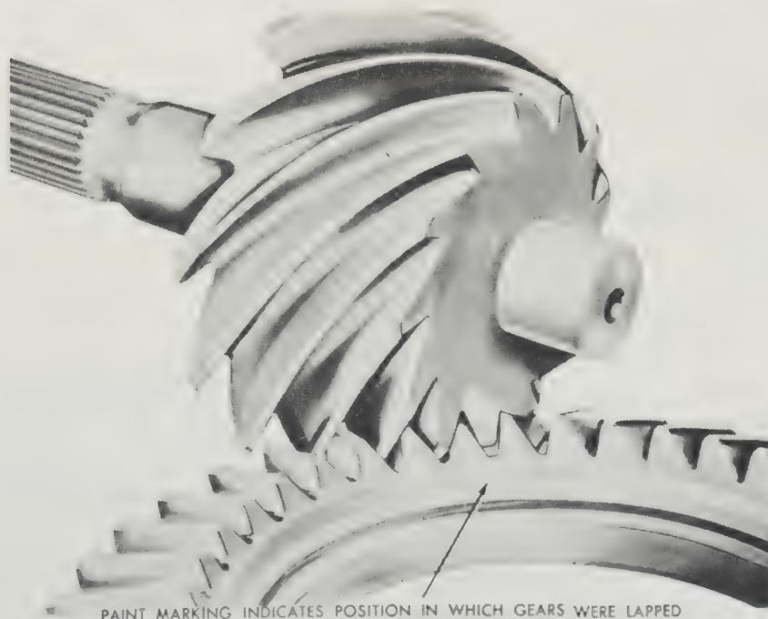
Fig. 8.10. Crownwheel and pinion indexing marks (Sec. 8)
