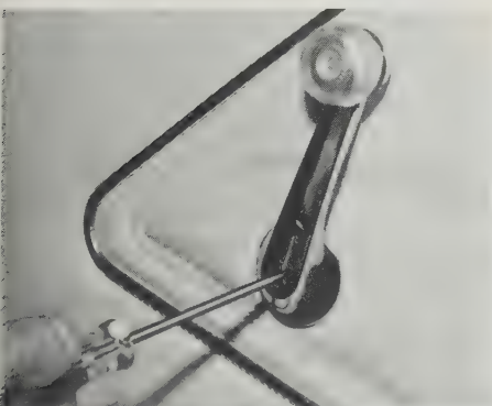
13.3A Removing window winder retaining screw
