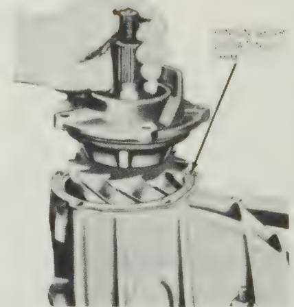
Fig. 8.9. Refitting the pinion gear and retainer (Sec. 8)
