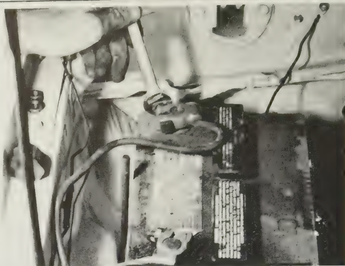
2.1 Removing battery terminal
