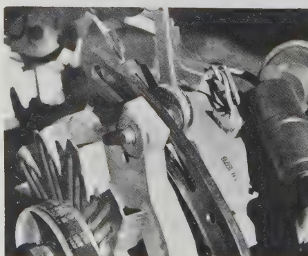
5.14 Slackening the alternator adjusting bolt
