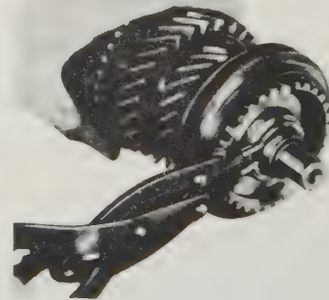
Fig. 6.9. Removing the front output shaft snap-ring (Sec. 6)
