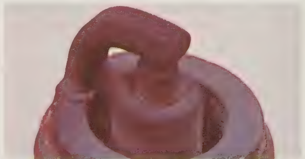
Carbon fouling. Dry, black, sooty deposits. Will cause weak spark and eventually misfire. Fault: over-rich fuel mixture. Check: carburettor mixture settings, float level and jet sizes; choke operation and cleanliness of air filter. Plugs can be re-used after cleaning
