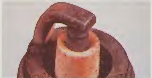
Overheating. Electrodes have glazed appearance, core nose very white – few deposits. Fault: plug overheating. Check: plug value, ignition timing, fuel octane rating (too low) and fuel mixture (too weak). Discard plugs and cure fault immediately
